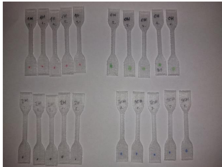
Figure 2. FDM 3D-printed PMMA specimens with test designations.
